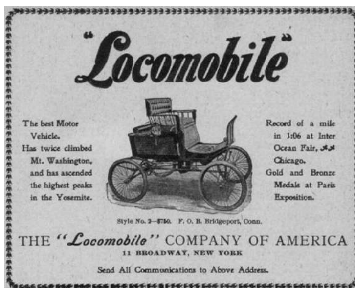
Fig. 1 – The best selling 1901 locomobile, a steam powered “Horseless Carriage” [6]
